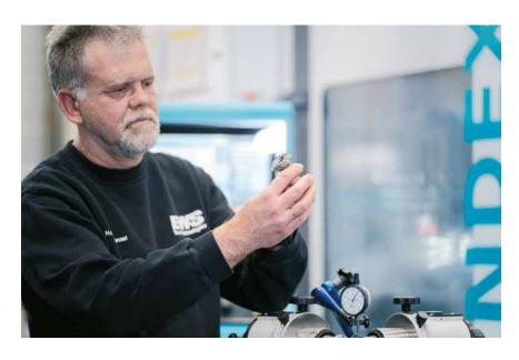
Left: The bevel gears that have just been machined are tested on a gear rolling tester machine alongside the INDEX G220. (Photos: FWS)
