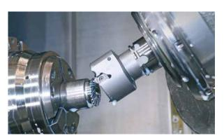
Bevel gear hobbing: the R and G-series INDEX turn-mill centers are particularly suitable for this gear cutting technology owing to their excellent static, dynamic, and thermal properties.
